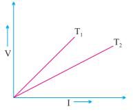
Ans. Slope of  $T_1$  is large, so  $T_1$  represents higher temperature as resistance increases with temperature for a conductor
