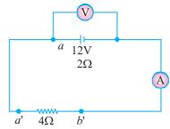
37. In the circuit shown, the reading of voltmeter is 20V. Calculate resistance of voltmeter. What will be the reading of voltmeter if this is put across 200 $\Omega$  resistance? **Ans.** R<sub>V</sub> =150 $\Omega$ ; V =  $\frac{40}{3}$  V
