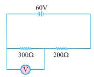
38. For the circuit given below, find the potential difference b/w points B and D.Ans. 1.46 Volts
